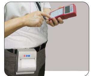
work as a mobile printer with handy terminal
